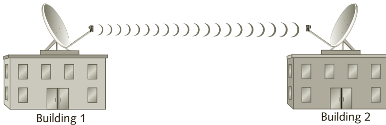
Figure 4-22 Point-to-point link using directional antennas
