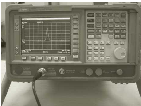
Figure 4-24 Spectrum analyzer showing amplitude (vertical size of on-screen graph) and bandwidth used by signal (bottom of on-screen graph)
