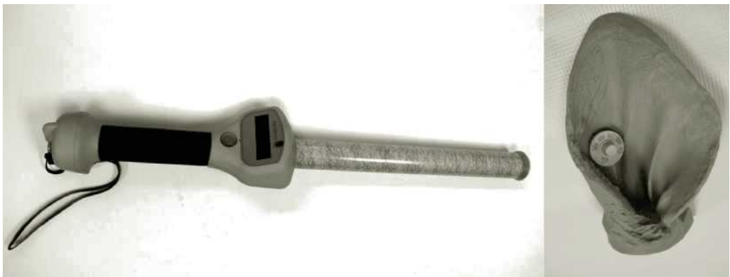
Figure 11-5 LF RFID wand reader and tag used in animals for tracking
