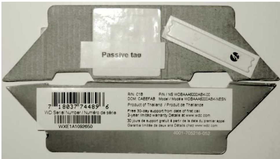
Figure 11-4 A passive and a 1-bit tag affixed to inside of the bottom flap of a product package (label shows barcode on the opposite flap for the same product)
