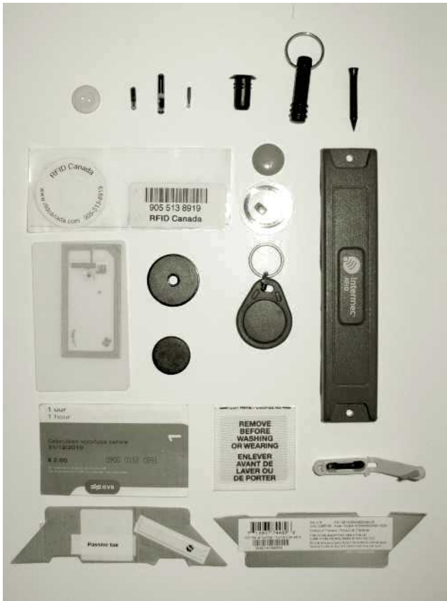
Figure 11-7 RFID tags are available in many shapes and sizes, for different applications
