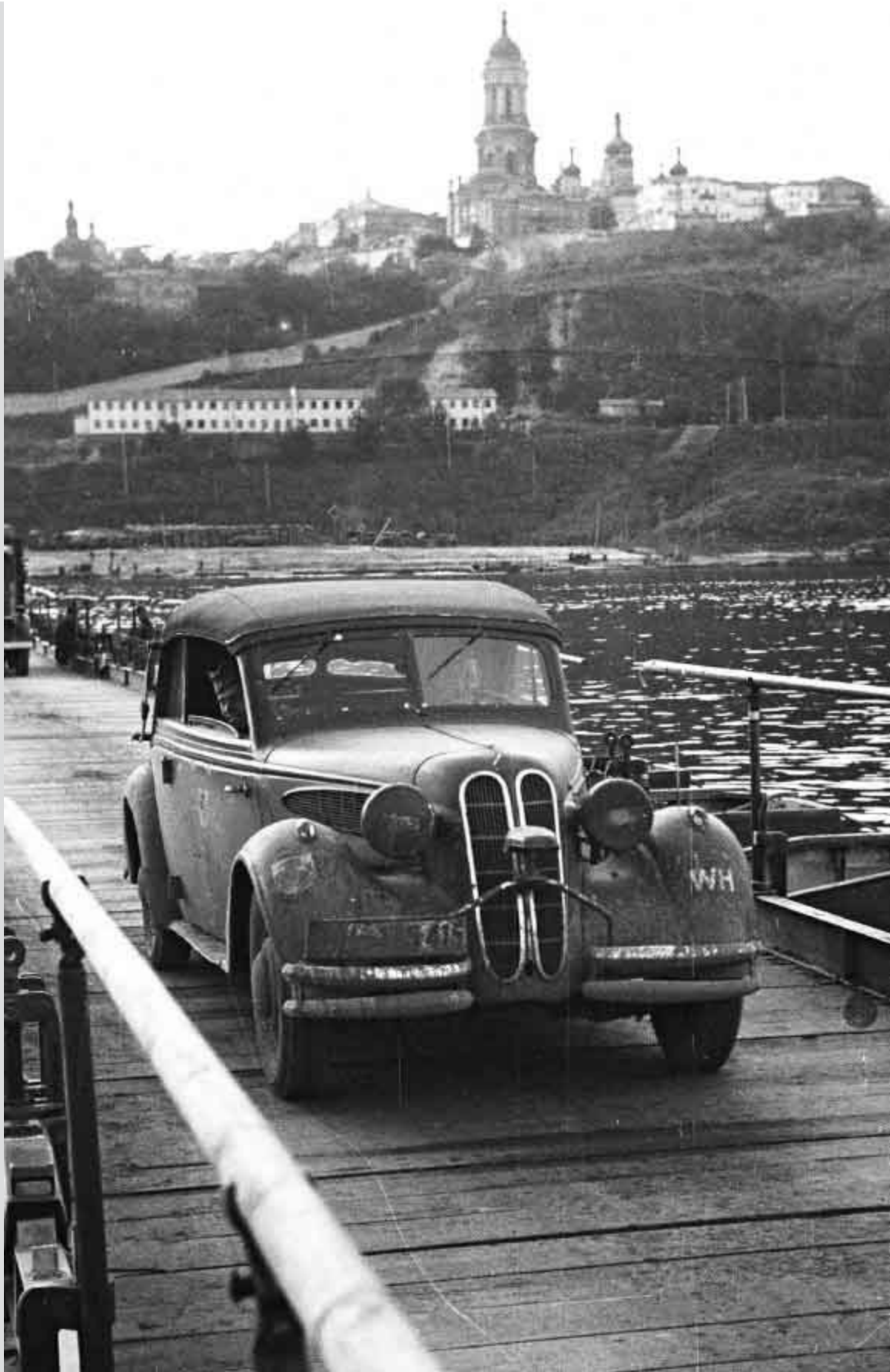
BMW 326 Cabriolet. Powered by a 50-hp, six-cylinder engine, this medium-sized civilian cabriolet, with its characteristic two-part bumper, was manufactured from 1936 to 1941.
