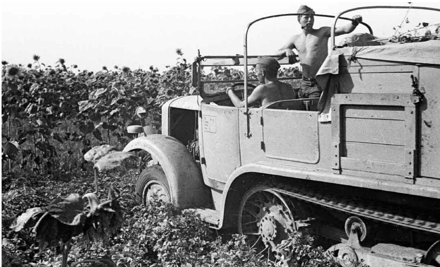
A French Unic Kégresse P107 half-track crosses a field of sunflowers. The Germans discovered in their first Soviet winter that sunflower oil was a superior acid-free alternative to their own lubricants, which froze in sub-zero temperatures. Enormous volumes of sunflower seeds and oil were also shipped to Germany for domestic use.
