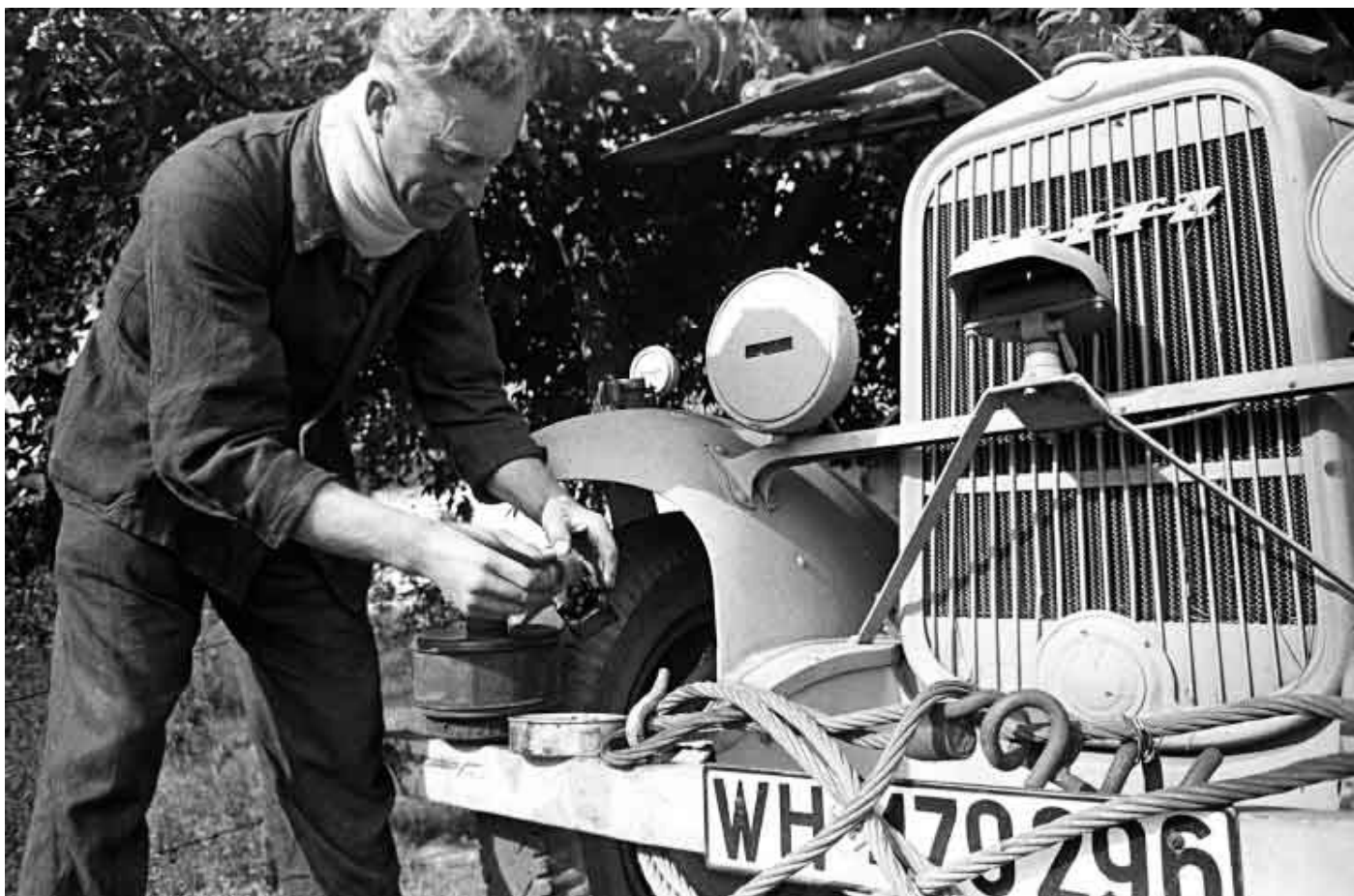
Cleaning the carburetor from an early model Opel Blitz with the air cleaner off to the side. An Operational Report
