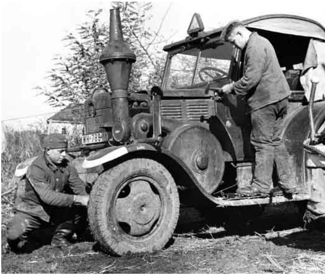
Top and above: A Lantz Eil-Bulldog type HR9 D2531. Easy to maintain with few moving parts, the tractor's single cylinder hot bulb 55-hp engine could run on a variety of different fuels. More than 2,400 examples of this model Bulldog were produced from 1937 to 1944.
