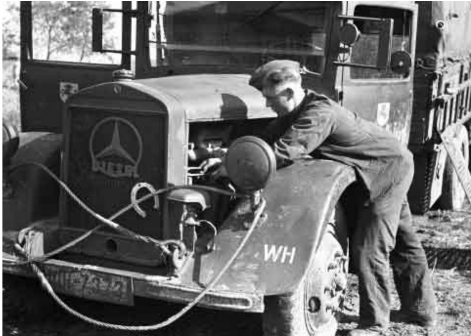
Top and above: Engine maintenance on a Mercedes-Benz L 1100 truck. These 1.1-ton vehicles were manufactured from 1932 to 1937. Emblazoned with the word 'diesel' on the radiator, Daimler-Benz at the time believed their compression-ignition engines were the benchmark of contemporary design and production.
