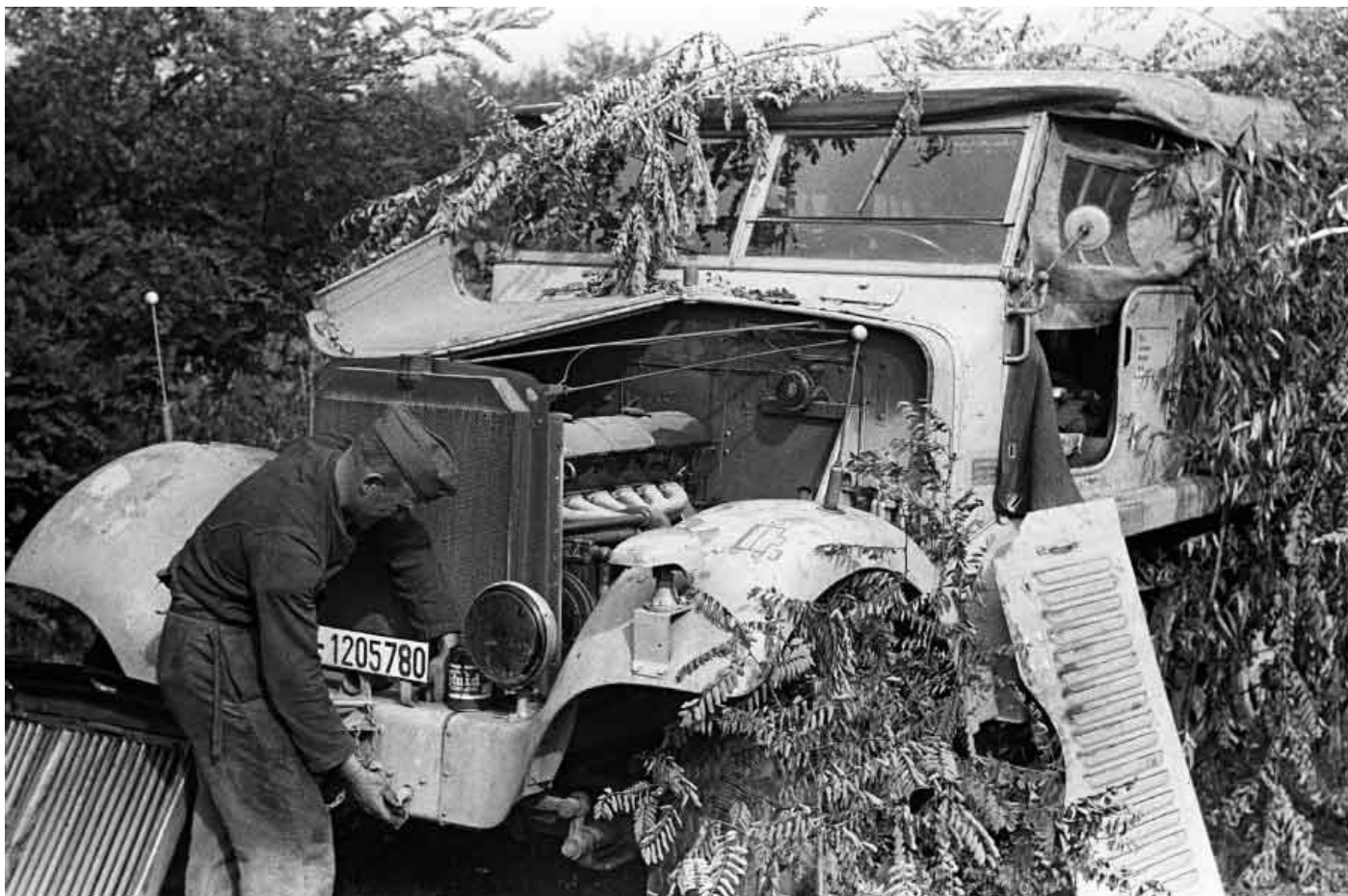
Engine maintenance on a heavily camouflaged Sd. Kfz. 6 half-track. The tactical symbol behind the Nachtmarschgerät signifies the vehicle belonging to a Fernsprechkompanie (Motorized Telephone Company).
