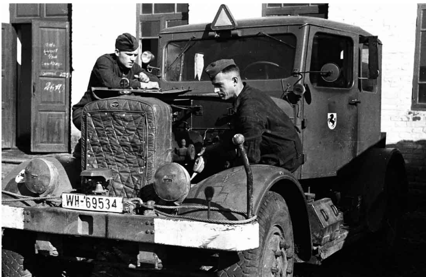
Servicing a Hanomag ( Hannoversche Maschinenbau AG ) SS 100 tractor. This military version of a 95-hp civilian
