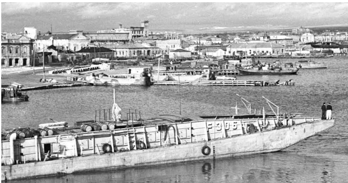
The Marinefährrahm (naval ferry barge) was a landing craft developed for the aborted 1940 invasion of England: Operation Seelöwe (Sea Lion). A total of 720 of these craft were built. MFP 306 was commissioned at Gollnow Shipyard, Stettin, on 19 June 1941. Assigned to the 3 Landungsflottille (3rd Landing Flotilla), this lighter was sunk by a bomb hit on the engine room at Kamysch-Burun, south of Kerch, on 30 November 1943.
