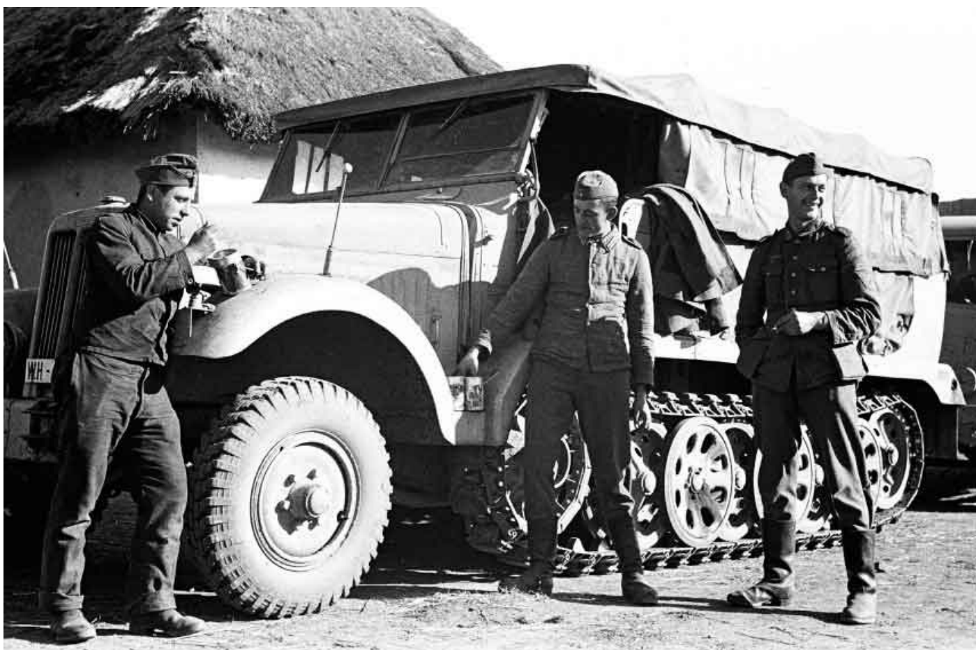
Top and above: These Sd. Kfz. 6 half-tracks show the evolution of paint schemes, from the early Dunkelgrau (dark grey) to the later Dunkelgelb (dark yellow), introduced in October 1942. As well as blending camouflage colours, a water-based white paint was also used during the winter snowfall.
