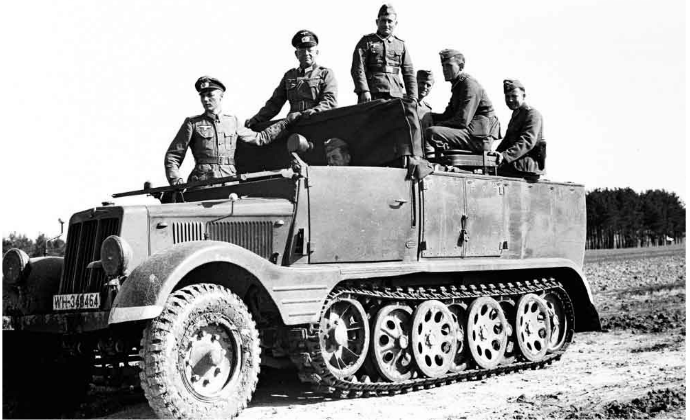
Top and above: The 3-ton leichter Zugkraftwagen Sd. Kfz. 11 light half-track vehicle was built from 1938 to 1945. A range of body types ranged from soft-skin to fully armoured. Regardless, these prime movers were costly and over-engineered for their primary role.
