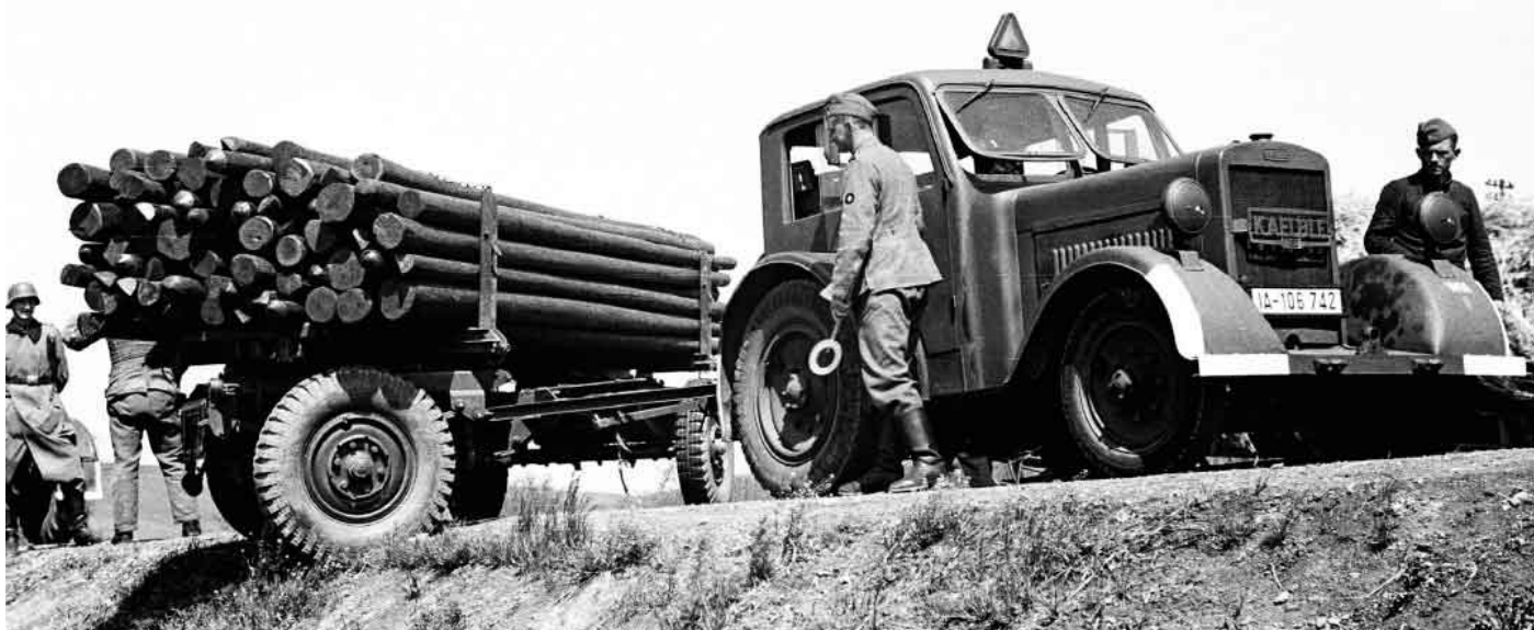
Jackknifed. A Sd.Ah. 21 trailer carrying telegraph poles and towed by a Kaelbler Z 4 G 110 tractor.
