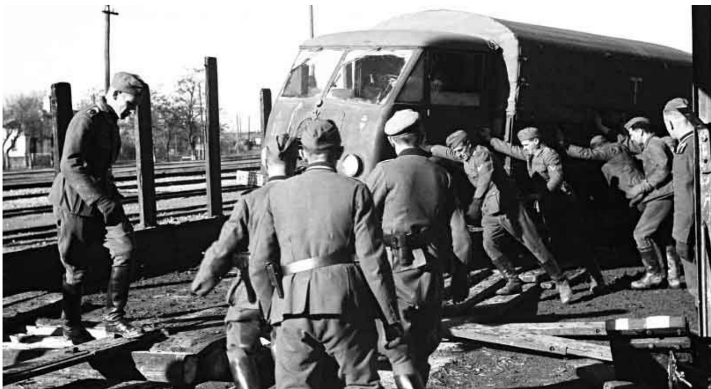
A French Matford V8-F917-F997WS truck is pushed into position on a flatbed carriage. Regulations stated that 'motor vehicles and tanks should be wedged in especially tight and lashed down with cables in order to prevent them from sliding.' Batteries were removed in cold weather and stored in heated passenger cars, and radiators were covered to prevent freezing in extreme cold.
