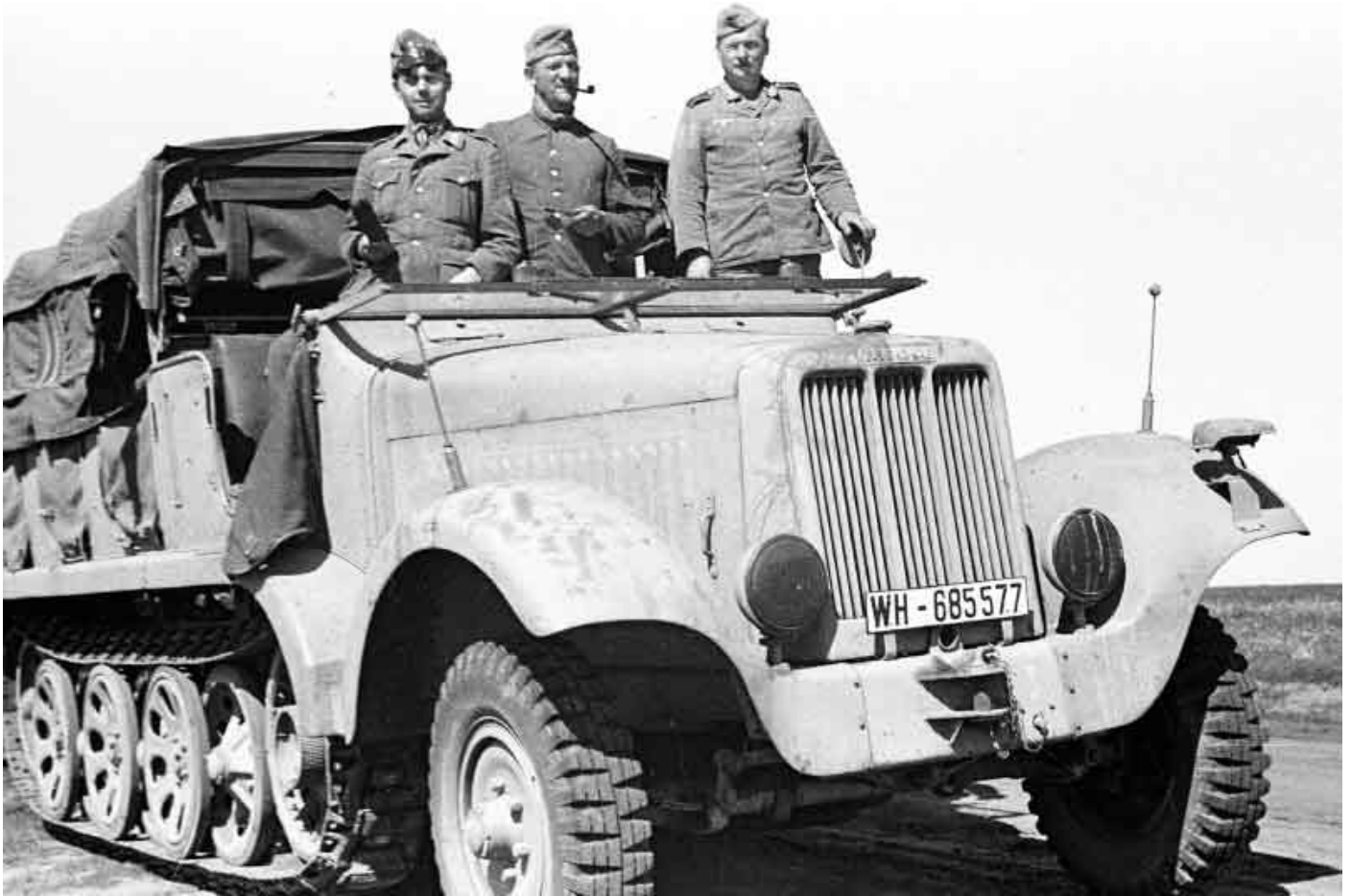
This Mittlerer Zugkraftwagen Sd. Kfz. 6 type BN9/9b medium half-track was built by Büssing-NAG. Note the Kfz-Nachtmarschgerät (night driving device) on the front left mudguard. Introduced in 1939, this helmet-shaped device directed light ahead of a vehicle at night that was not visible from the sky or to ground observers.
