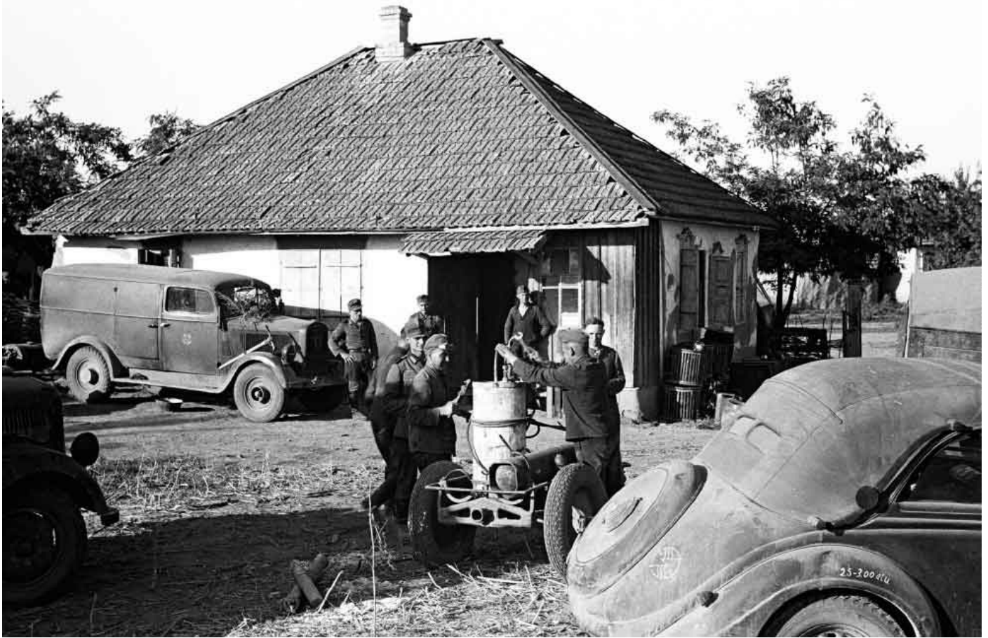
Oxyacetylene equipment is wheeled on a makeshift single axle trailer. The car in the foreground is a BMW 326; the truck in the rear is an Opel Blitz 2, 0-12 1-ton truck. After General Motors acquired Opel in 1931, many components were practically identical to Chevrolet light duty trucks manufactured in North America.
