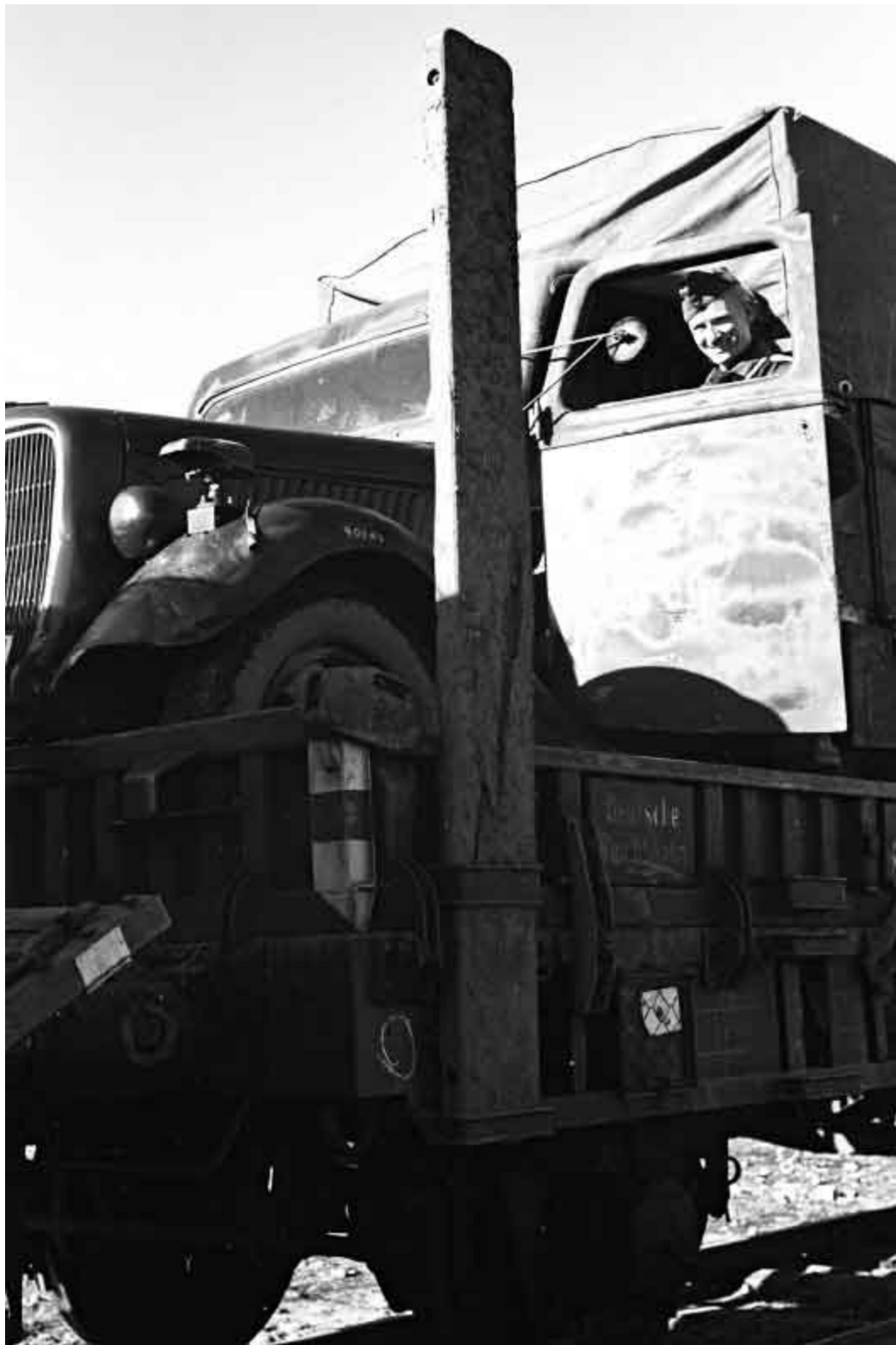
The 3-ton Ford V8-51, successor to the Ford BB, was manufactured in Germany from 1937 to 1939.
