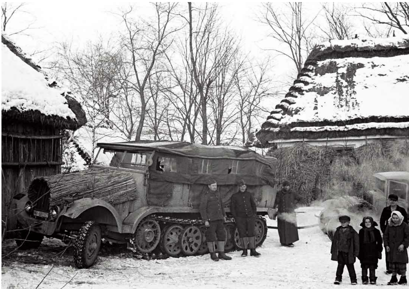
A Sd. Kfz. 6 half-track, with improvised engine insulation to prevent the radiator freezing, tows an engineless truck outside a billeted izba (traditional dwelling). Writing in Signal , Erich Neumann observed that ‘No soldier any longer speaks of what it was like in the dry dust of summer swarming with myriads of insects or in the grim and boundless mud of autumn, for the snow lying yards deep, beneath which the remains of the victims of that time sleep, the skeletons of the dead horses and the scrap metal of wrecked lorries provides sufficient new cares for topics of conversation in the evenings in the Soviet billets.’
