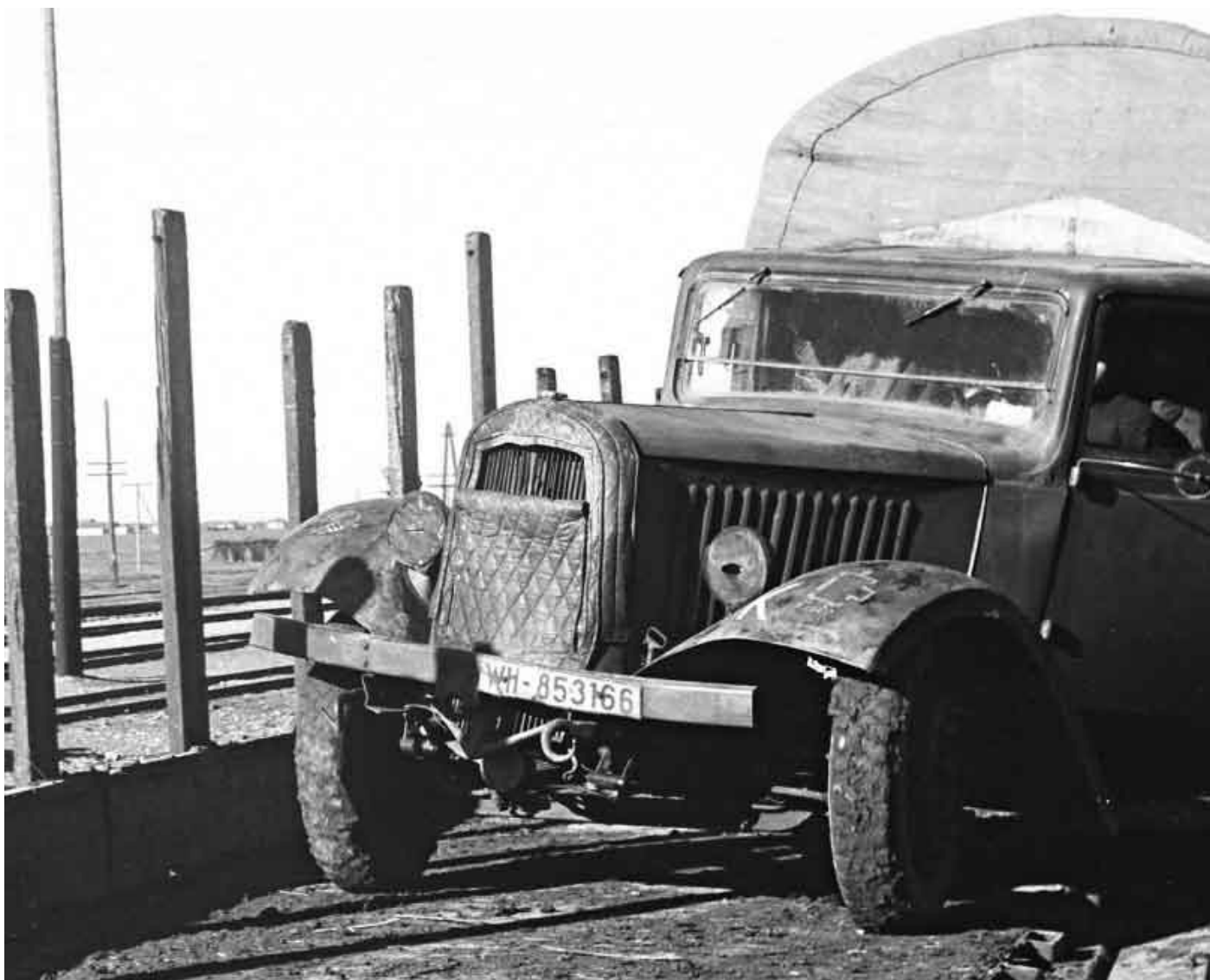
The Citroen Type 45 U saw widespread use on the Eastern Front. Some 18,500 of these 73-hp French trucks were manufactured for the Wehrmacht from 1941 to 1944. Note the cold weather radiator cover.
