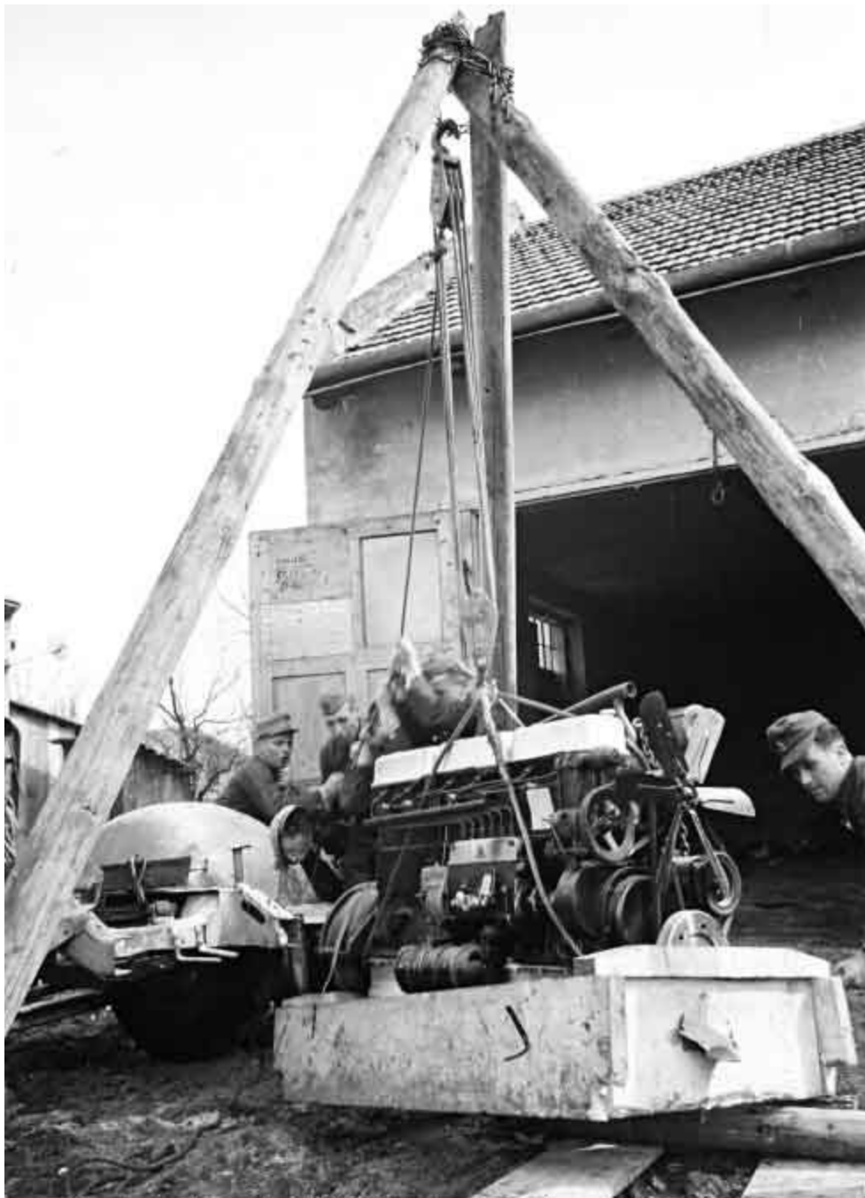
A replacement engine is hoisted using a block and tackle in a makeshift field workshop. Forward overhaul, unlike the opening campaigns of the war, became a major problem during the protracted Soviet campaign. Workshops for major repairs during the opening months of the invasion remained to the rear in Poland and Germany.
