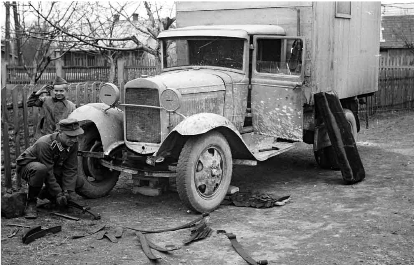
Fixing the broken leaf spring suspension of a Soviet GAZ-AA. These basic vehicles were simpler and generally more reliable than their complex Western European counterparts. German mechanics, however, faced the challenge of fixing numerous different models, especially as the war progressed and greater numbers of captured and requisitioned civilian vehicles were pressed into service.
