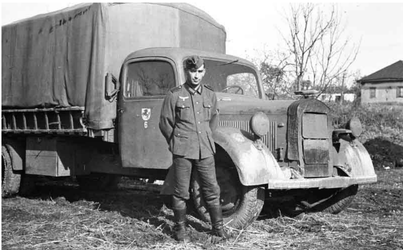
Mercedes-Benz L 3000 S. Note the bomb emblem in place of the Gottlieb Daimler's iconic 3-pointed star. Approximately 16,000 examples of this 3-ton vehicle were produced from 1938 to 1944. It was not as popular with troops who preferred the more reliable Opel Blitz (Lightning) 3-ton series with its superior cross-country performance.
