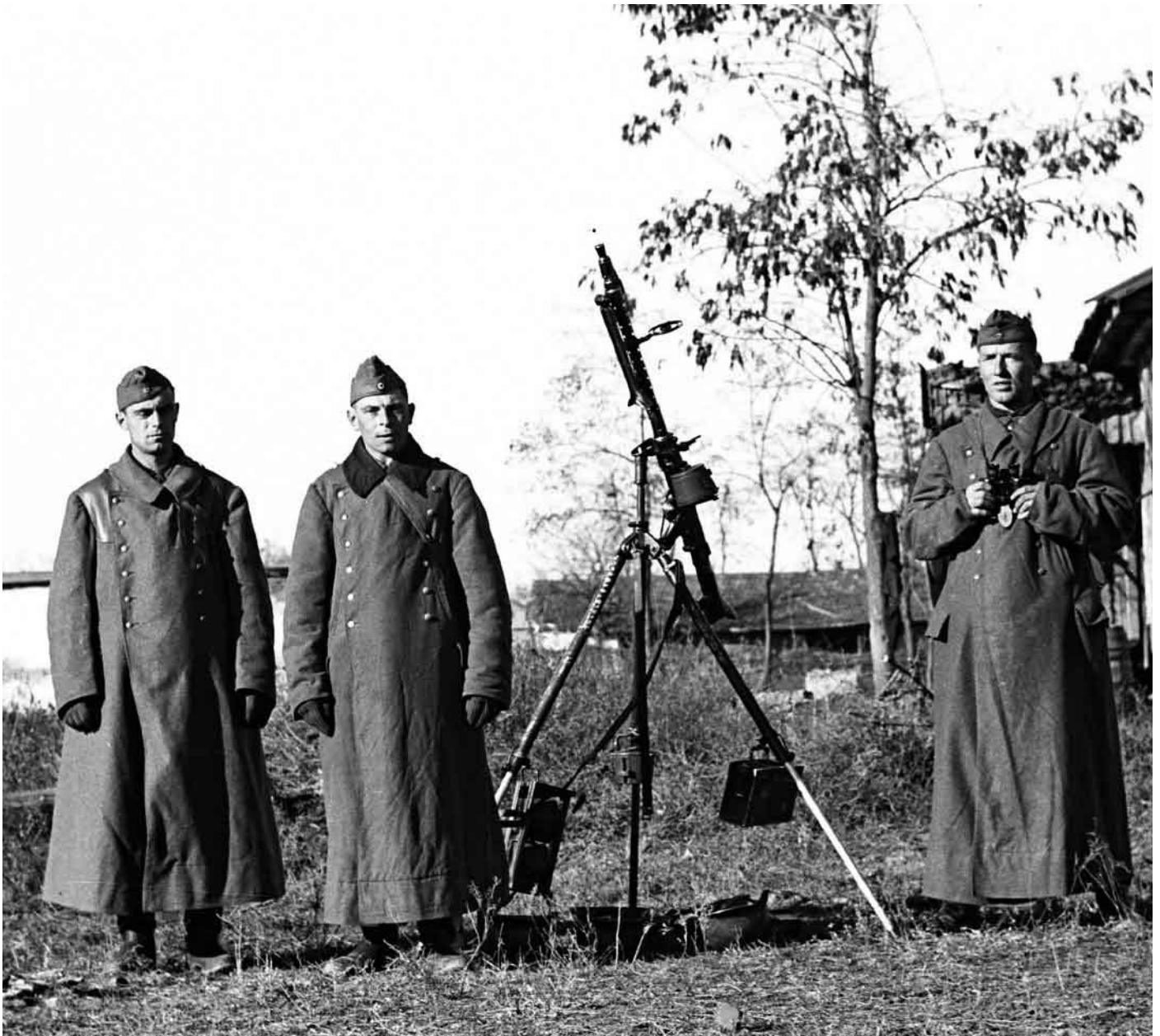
The recoil operated, air cooled MG34 machine gun was a versatile weapon that operated on a number of different mounts and with different optical sights. Mounted on a tripod for anti-aircraft defence, this gun has a Gurtrommel 34 fifty-round basket magazine with two extra Patronenkasten 41 ammunition cans at the ready.
