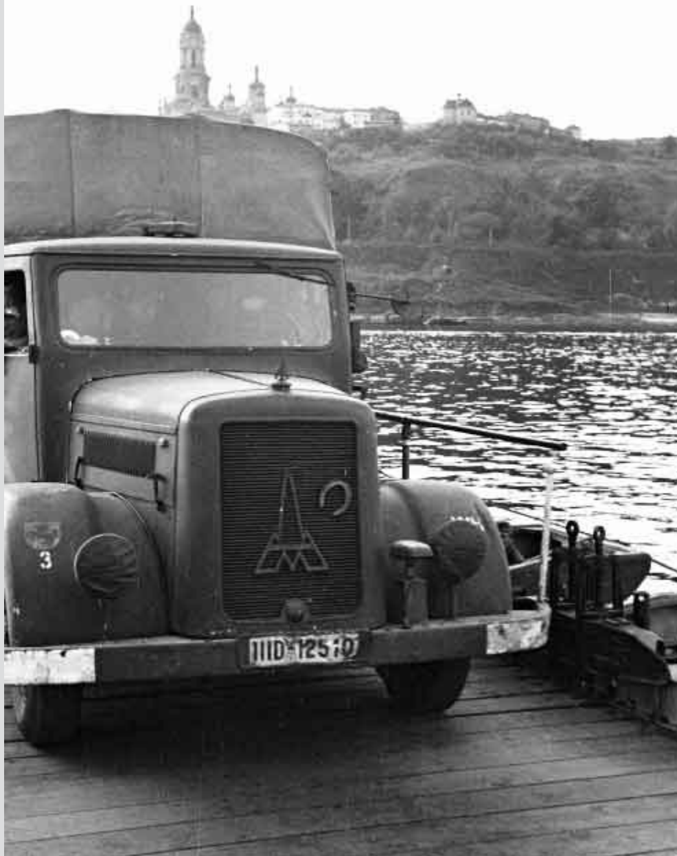
Magirus L 235. Powered by 85-hp four-cylinder Deutz diesel engine, 2,070 of these trucks were manufactured from 1937 to 1940.
