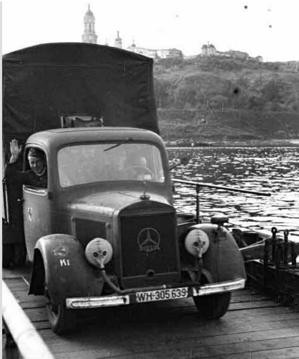
Mercedes-Benz trucks, either type L 1500 or L 2000. Note the stylized Soviet gas mask headlight covers.
