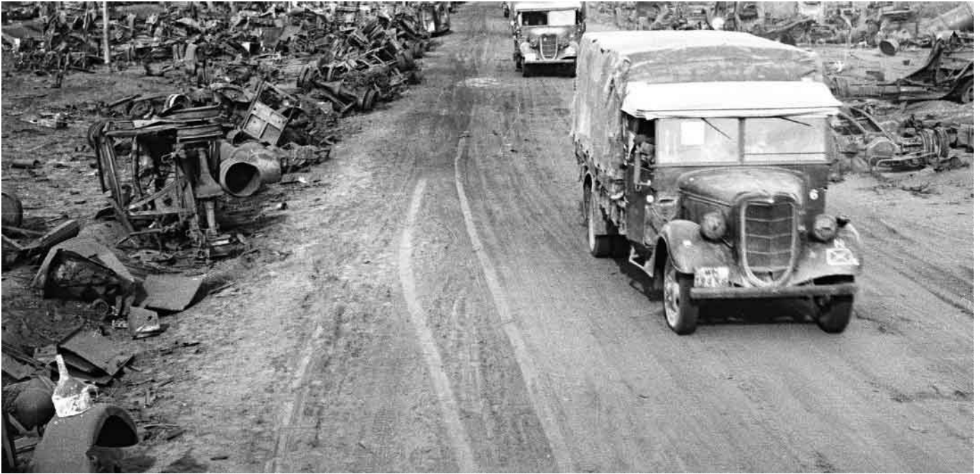
A column of Ford V8-51 trucks on a road lined with Red Army wreckage. The tactical symbol 'N' on the vehicle's fender stands for Nachschub (supply unit).
