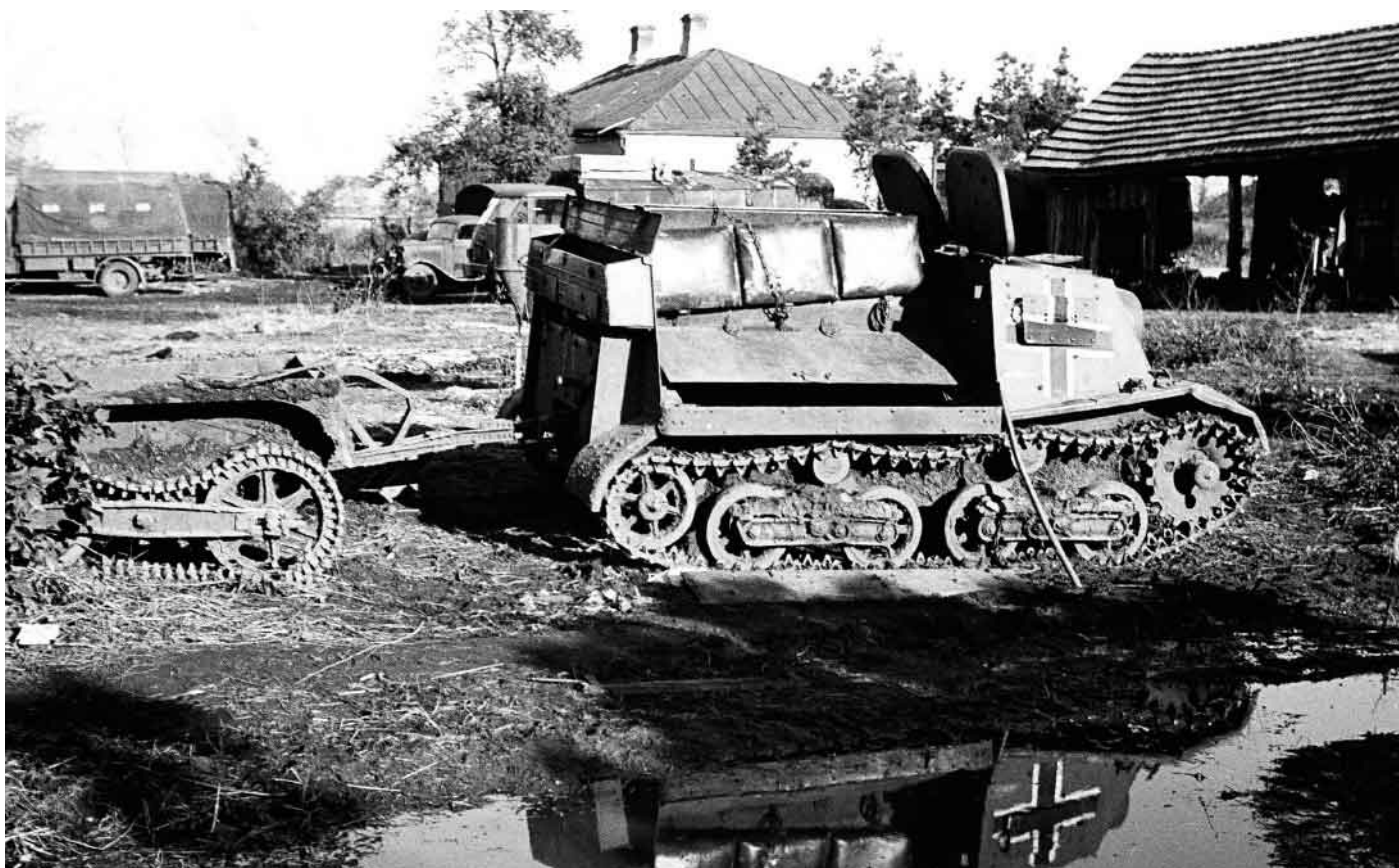
A Soviet T-20 Komsomolets light artillery tractor under new ownership. Germany, Romania and Finland all used captured T-20s with some German examples armed with a 3.7-cm Pak 35/36 antitank gun. This vehicle is shown
