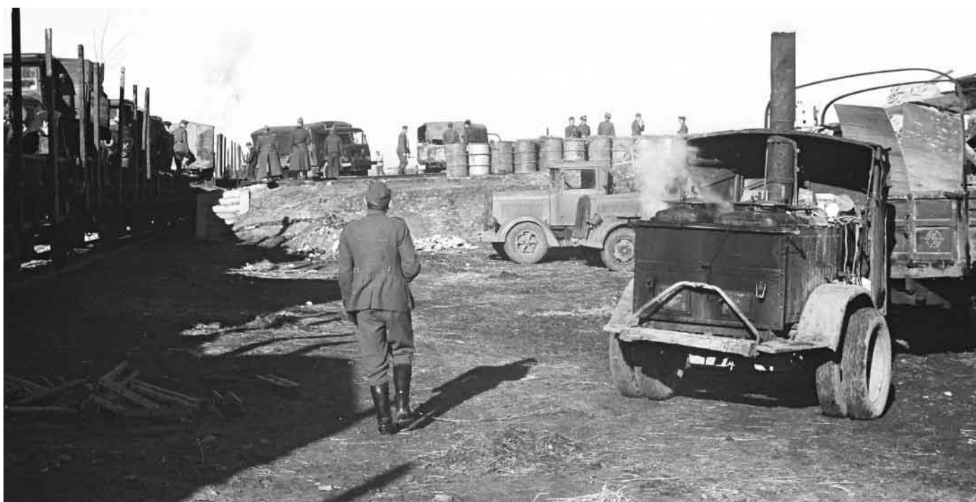
This steaming Feldküche (field kitchen) is a captured Russian type KP -3 -37(r): KP = kuchnya polewaya (Russian for field kitchen); 3=three boilers; 37=Year of introduction; r=Wehrmacht abbreviation for captured Russian equipment. Note the trailer's height, which presented problems when serving meals, and dual tyres.
