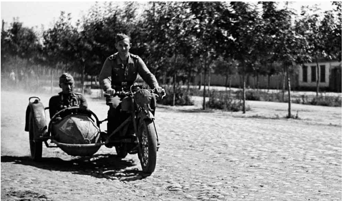
A German motorcycle with the distinctive Steib sidecar Nr28. A BMW designer sent to the Ostfront reported: 'we sought out the field repair shops, which operated in the most primitive conditions, directly behind the front line. There the machines were examined and reports on the troops' experiences were taken. My opinion was correct. The machines went under the liquid mud, which flowed over the motors by the bucketful and was sucked into the low-lying air filter, ruining it – the mud got into the motor, and often the oilpans no longer held oil, but only sand.'
