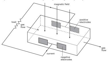
Magnetohydrodynamics. Magnetohydrodynamic generator.
