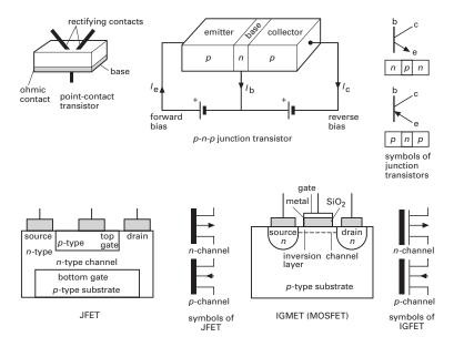
JFETs are made with both n-type and p-type channels.
