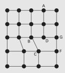
**Dislocation in a two-dimensional crystal.** The extra plane of atoms AB causes strain at bond CD. On breaking, the bond flips across to form CB. This incremental movement shifts the dislocation across so that the overall effect is to slide the two planes BDG and CF over each other.
