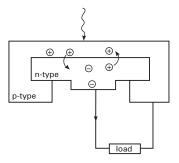
Solar cell. A silicon p-n junction.
