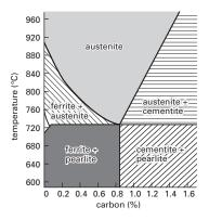
Steel. Phase diagram for steel.
