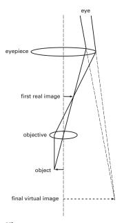
Microscope. Compound microscope.
