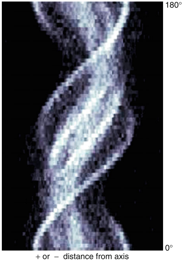
Fig. S.2 Sinogram from a SPECT scan of a phantom that includes among other things two off-center hot spots . As the angle of viewing increases (from bottom to top of figure), these appear, when viewed by detectors, at different distances (horizontal in this figure) from the centerline. With this progression of the viewing angle through 180^\circ , the hot spots each trace a sine-wave (the two outermost spirals) from bottom to top of the sinogram. Other off-axis regions of activity concentration closer to the axis are also seen here. Also it is noticeable: how a limited number of discrete quantitative values from reconstruction are displayed by a gray scale within square pixels; and how the original display software provides fuzzy edges for these in its chosen resolution. (Reprinted with permission from the Wikimedia Commons repository of the Wikimedia Foundation from file, Spect_sinogram_360.jpg , http://commons.wikimedia.org/wiki/ . Accessed 28 September 2011)
