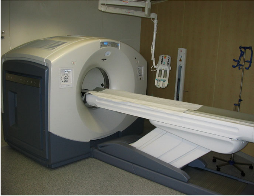
Fig. P.4 PET/CT showing the gantry housing the detectors (the left center ) and the moveable bed (the right foreground ). As the bed moves the patient into the gantry interior a portion of his body is scanned, the axial length of which is the field of view located within the gantry. In the whole body scan , the bed pauses at successive positions while sections are scanned. Both the PET and the CT scans can take place while the patient remains on the bed (Reprinted with permission from the Wikimedia Commons repository of the Wikimedia Foundation from file, 16slicePETCT.jpg, http://commons.wikimedia.org/wiki/ . Accessed 28 September 2011)
