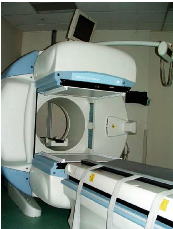
Fig. S.1 SPECT/CT showing its gantry in the rear holding the two gamma cameras that rotate and then stop for scans of the patient positioned on the bed in the lower foreground. The device does both a SPECT and a CT scan (Reprinted with permission from the Wikimedia Commons repository of the Wikimedia Foundation from file, HybridSpectCTScanner.png, http://commons.wikimedia.org/wiki/ . Accessed 28 September 2011)
