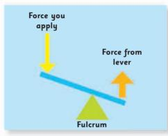
If the force you apply is twice as far from the fulcrum as the force the lever produces, the lever doubles the force.
