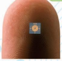
A silicon chip can be very small—less than 1/10 square in (1 cm<sup>2</sup>) and about 1/10 inch (1/2 a mm) thick.
