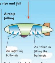
To descend back down to Earth, the ballonets are filled with the heavier air, making the airship sink.
