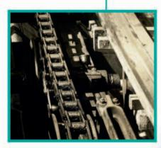
**Chain reaction** Roller-coaster cars don't have motors. They're pulled to the top of the first hill by a chain connected to a motor at the top.
