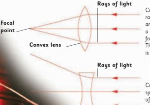
Convex lenses bend rays of light together and bring them to a point called the focus, or focal point. The lens in your eye is convex.
