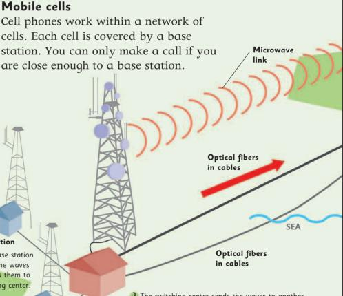
3 The switching center sends the waves to another switching center, either as microwaves or through optical fibers in cables under the ground or sea.
