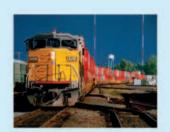
Most freight trains are powered by diesel electrics.
