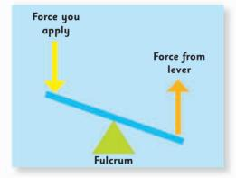
If the force you apply is the same distance from the fulcrum as the force the lever produces, the two forces are equal.
