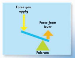
If the force you apply is three times as far from the fulcrum as the force the lever produces, the lever triples the force.
