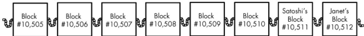
Figure 2-13: Bitcoin miners Crowley and Satoshi find a block at the same time, creating two copies of the blockchain. The resolution to the forked blockchain occurs when Satoshi's version of the blockchain adds another block before Crowley's, and Satoshi receives the reward.
