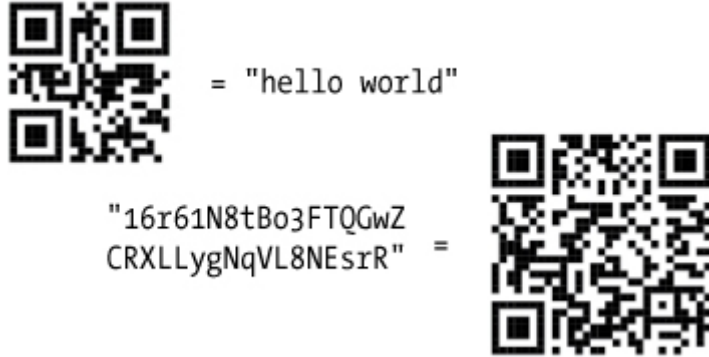
Figure 2-1: QR codes can be used to represent arbitrary data. They are easy to scan with smartphones and so are convenient for sharing the long strings of characters used for Bitcoin addresses.
