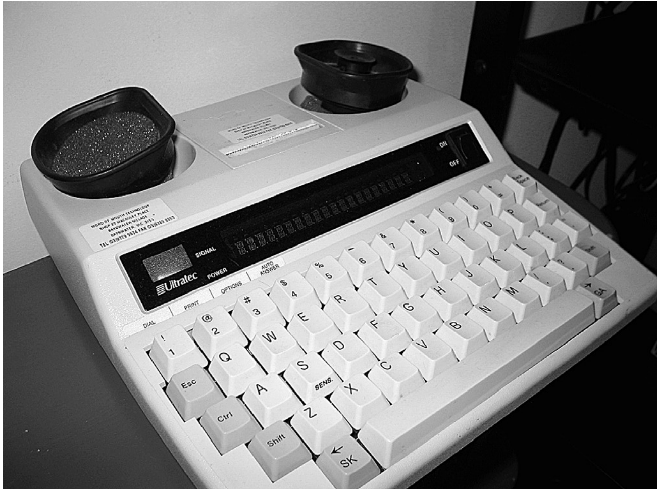
A Miniprint 425 telecommunication device for the deaf. The acoustic coupler on the top is for use with telephone handsets, and a printer records the conversation. The specific GA and SK keys allow for speedier use of common abbreviations. It has become a widespread belief that access for the deaf to telecommunications and information is as vital as any other civil right.
