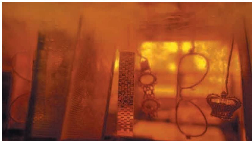
Figure 13.8 A less expensive metal can be silver-plated to produce an attractive and corrosion-resistant surface. The object to be plated is connected to a circuit as the cathode. It is suspended in a solution containing silver cyanide. The silver ions are attracted to the cathode, where they combine with electrons and become solid silver atoms that remain permanently attached to the surface of the cathode.
