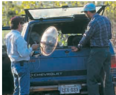
Figure 9.40 A parabolic reflector around a microphone focusses sounds and allows distant noises to be clearly recorded.
