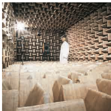
Figure 9.41 An anechoic chamber that is literally “without echo” yields sound power reduction that follows the inverse square law ( 1/r^2 ).
