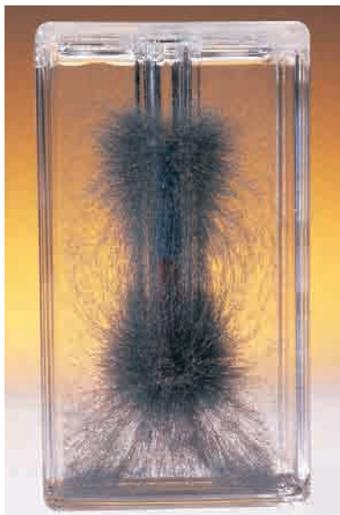
Figure 14.10 A suspension of iron filings in glycerine is used to demonstrate the third dimension of a magnetic field.
