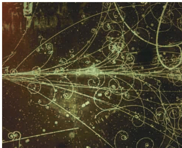
Figure 4.21 Particles of different mass and charge produce different trajectories. You cannot see the particles but you can see their tracks.
