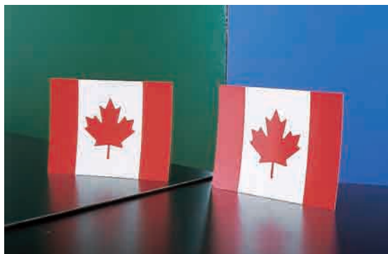
Figure 10.8 The image of the flag is the same size, is upright, and is the same distance behind the mirror as the flag is in front of it. However, if you hold a screen behind the mirror where the image appears to be, no light from the flag is able to reach the screen. The image formed by any plane mirror is a virtual image.
