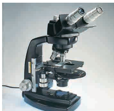
Figure 12.22 The lens arrangement of a microscope is similar to that of an astronomical telescope. In a binocular microscope, the light from the objective lens is split in two by prismatic mirrors and directed to the eyepiece lenses.
