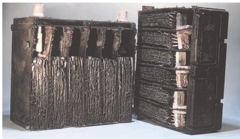
Figure 13.23 A chemical reaction separates electric charge creating a potential difference between the terminals. Internal resistance within the battery reduces the amount of voltage available to an external circuit.
