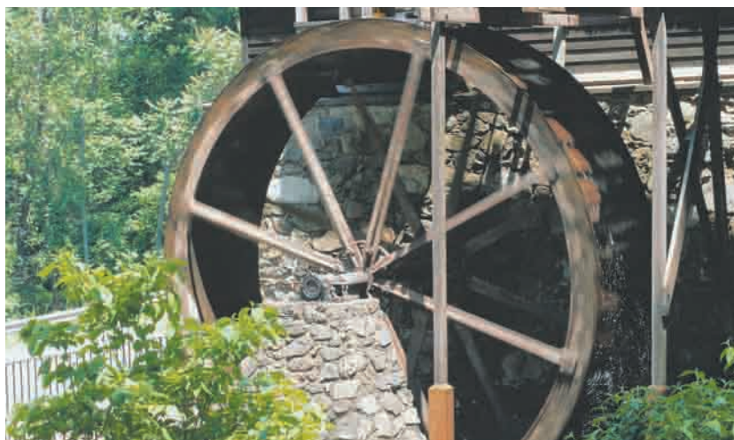
Figure 5.20 Gravitational potential energy is stored in the water. When the water begins to fall, it gains kinetic energy. As it falls, it turns the wheel, giving the wheel kinetic energy.
