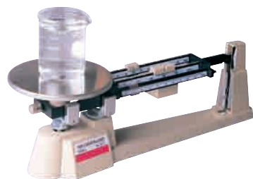
Figure 15.14 The motion of the arm in the triple-beam balance results in eddy currents in the plate at the end of the arm. By Lenz's law, the energy to cause the eddy currents must come from the kinetic energy of the arm, damping its motion.
