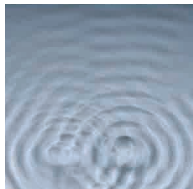
Figure 7.26 A series of antinodes run along the vertical line up the centre. The lines spreading out beside the antinodes are formed by nodes.
